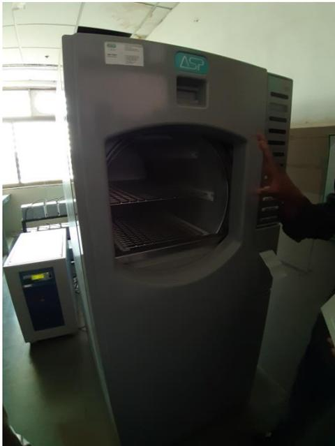
First the  $H_2O_2$  is inserted into sterilizer where it is heated at high temperature and is converted to gas and after that this gas is surrounded by an strong electromagnetic field as a result it becomes a plasma. This plasma is then dispersed in a sterilizer chamber which oxidizes the germs and micro-organism on a load as result it gets killed.
